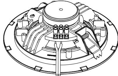
Connect the wires coming from the amplifier to the terminal block connector on the rear of the loudspeaker.
