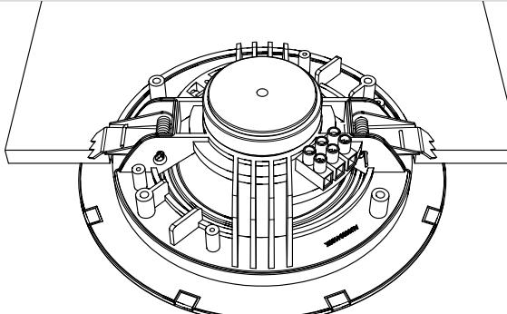
Insert the speaker through the provided ceiling cut-out, make sure the spring loaded mounting arms are behind the clamping surface and release them. The ceiling is clamped between the mounting arms and the speaker baffle and is installed correctly.
