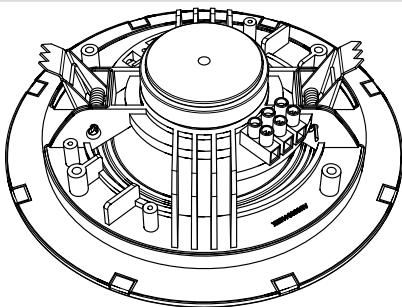
Bend the spring loaded mounting arms inwards by pushing them by fingers, making them fit through the provided ceiling cut-out.
