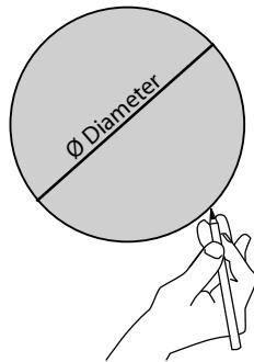
Cut a hole on the desired mounting location in the ceiling. Make sure the dimension is matching the cut-out measurement for the installing loudspeaker
