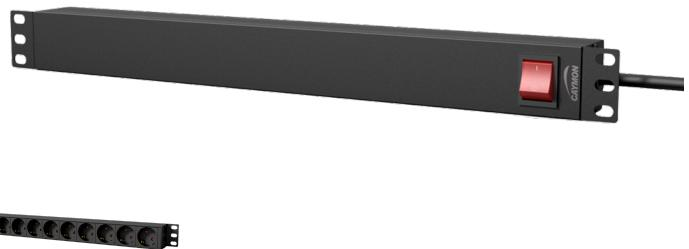
The PSR1x9Gx are 19" power distribution unit, compliant to the ANSI/EIA RS-310D, DIN41491 and IEC60297 standards. They come in three different models, without a switch (PSR109G), with an illuminated switch on the socket side (PSR109GS) or with an illuminated switch on opposite of socket side (PSR119GS). The construction is made using black powder coated aluminum fitted with steel 19" mounting ears on each side.
