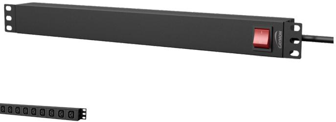
The PSR1x9Ex are 19" power distribution units, compliant to the ANSI/EIA RS-310D, DIN41491 and IEC60297 standards. They come in three different models, without a switch (PSR109E), with an illuminated switch on the socket side (PSR109ES) or with an illuminated switch on opposite of socket side (PSR119ES). The construction is made using black powder coated aluminum fitted with steel 19" mounting ears on each side.
