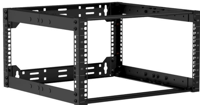
The OPR506A is an in depth adjustable professional and solid constructed open frame rack for 19" equipment compliant to ANSI/EIA RS-310D, DIN41491 and IEC60297 standards which is suitable for wall mounted or floor standing installation. It ensures maximum installation, connectivity and maintenance ease storing up to 6 units of 19" equipment.
