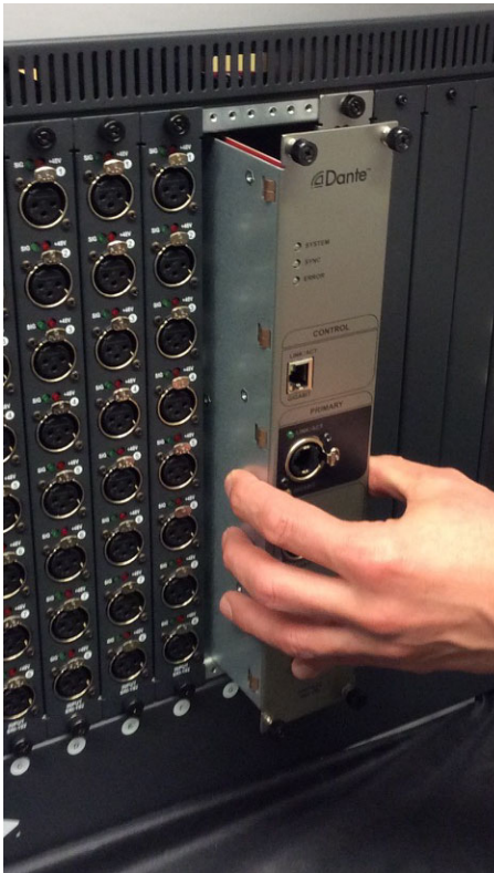
Figure 4. Sliding the card into a Stage 64 (shown at left) and a DNT-192 card aligned with the interior channel in a Stage 32 (shown at right)
