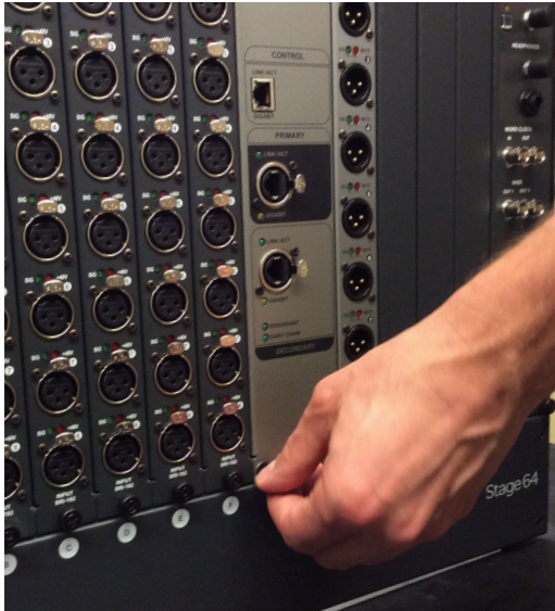
Figure 6. Tightening one of the four front captive thumbscrews (Stage 64 shown)
