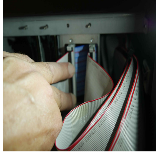
Figure 8. Connecting ribbon cable in a Stage 64 (shown at left) and Stage 32 (shown at right) Your installation may appear differently depending on the slots used for the DNT-192 card
