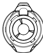
powerCON True1 AC Cable Input Connector
