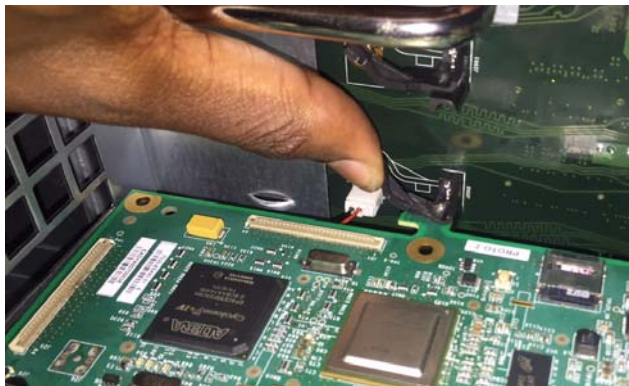
Lifting the tab on the retaining clip
