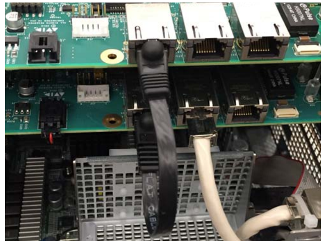
Ethernet cable connected between cards
