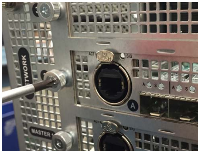
Tightening the exterior thumbscrew
